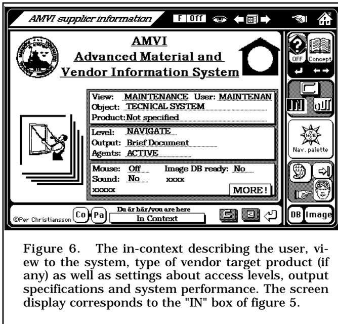
Figure 6. The in-context describing the user, view to the system, type of vendor target product (if any) as well as settings about access levels, output specifications and system performance. The screen display corresponds to the "IN" box of figure 5.
