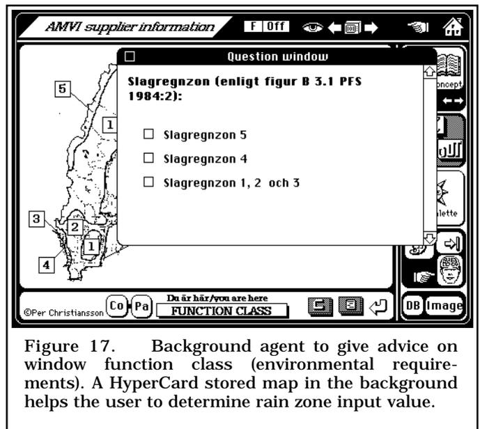
Figure 17. Background agent to give advice on window function class (environmental requirements). A HyperCard stored map in the background helps the user to determine rain zone input value.
