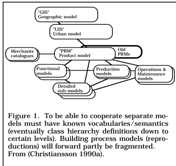
Figure 1. To be able to cooperate separate models must have known vocabularies/semantics (eventually class hierarchy definitions down to certain levels). Building process models (reproductions) will forward partly be fragmented. From (Christiansson 1990a).
