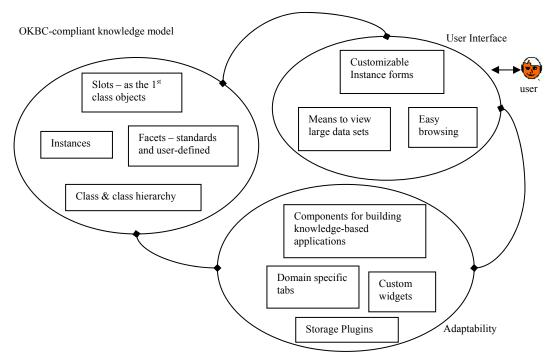
Figure 8.2: The component-based architecture of Protégé.
