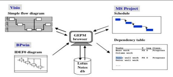
Figure 3.2: The GEPM Process Model enhanced with more modelling power compared with other methods available at one time. (Source: Karhu, 2001)
