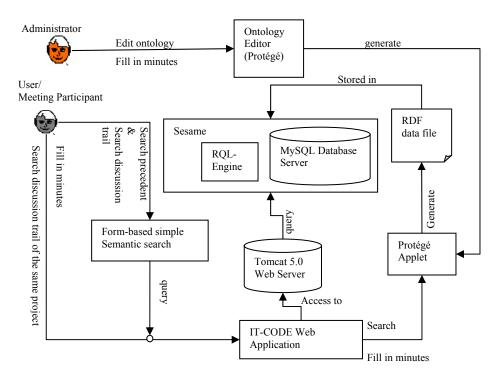
Figure 8.4 Architecture of the demonstrator.
