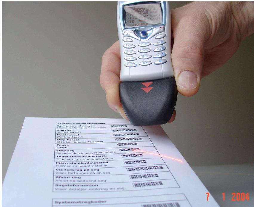
Figure 3 Ericsson T68i Mobile phone equipped with barcode reader scanning a laminated barcode sheet.
