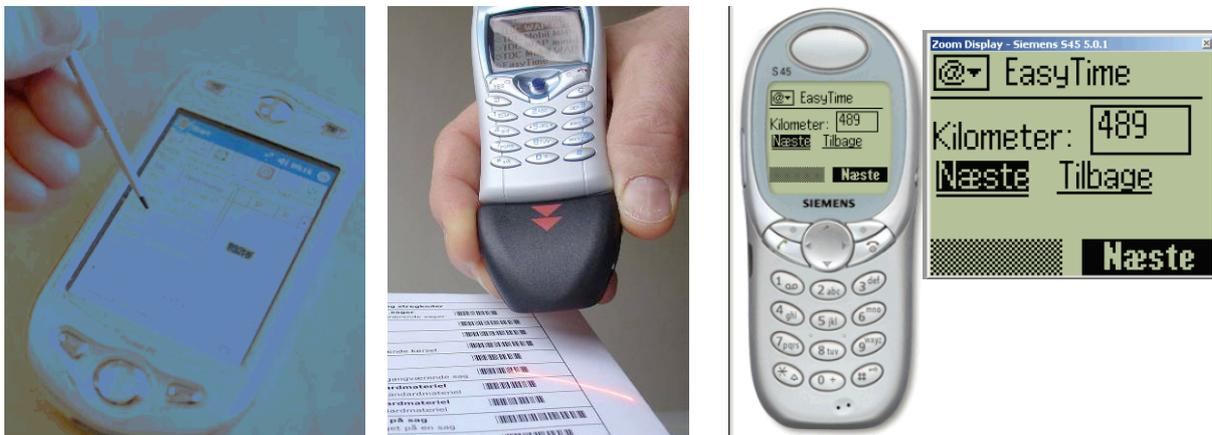
Fig 1 The three systems in test: PDA, mobile phone with barcode reader and ordinary mobile phone.
