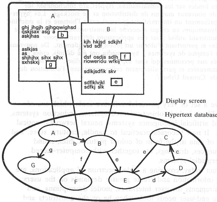
Figure 2. "The correspondence between windows and links in the display, and nodes and links in the database. In this example, each node in the hypertext database is displayed in a separate window on the screen when requested. The link named b in window A has been activated by a pointing device, causing a new window named B to be created on the screen and filled with text from node B in the database." (Source: Conklin, 1987.)
