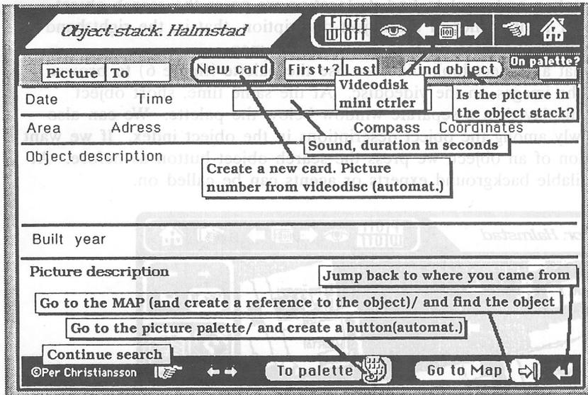
Figure 9. Layout of object descriptions with tools to build, search, and navigate.
